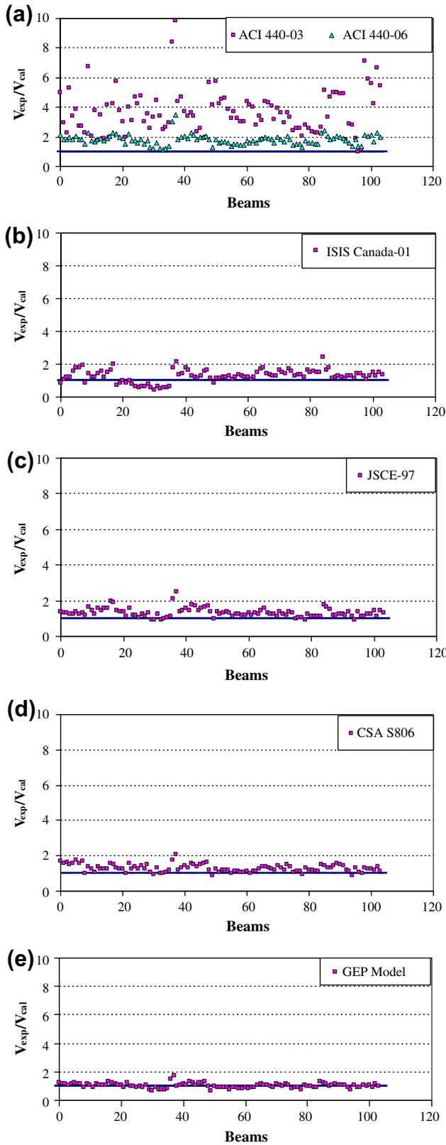
Fig. 7. (a–e) Performance of shear design equations in calculating shear capacity of FRP-reinforced concrete beams without stirrups.
