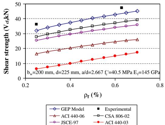
Fig. 11. Effect of the longitudinal reinforcement ratio ( $\rho_f$ ) on the shear strength of FRP-reinforced concrete beams without stirrups.
