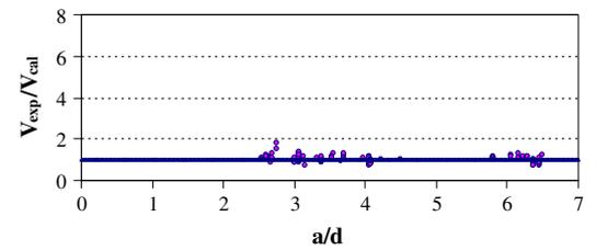
Fig. 10. Experimental to calculated shear strength versus shear span-to-depth ratio.
