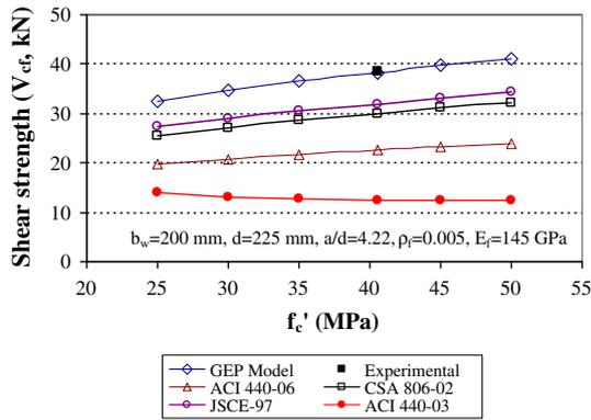
Fig. 12. Effect of the concrete compressive strength ( $f'_c$ ) on the shear strength of FRP-reinforced concrete beams without stirrups.
