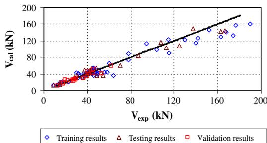
Fig. 6. Comparison of  $V_{cf}$  experimental shear strength results with the results of GEP model.
