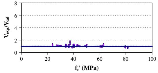
Fig. 8. Experimental to calculated shear strength versus concrete compressive strength.
