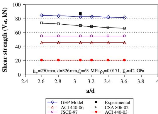
Fig. 13. Effect of the shear span-to-depth ratio ( $a/d$ ) on the shear strength of FRP-reinforced concrete beams without stirrups.
