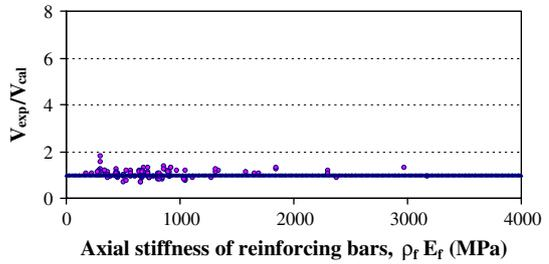
Fig. 9. Experimental to calculated shear strength versus axial stiffness of reinforcing bars.
