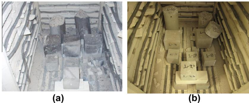
**Fig. 2.** Explosive spalling after heating at 600 °C for: (a) NVC2 and (b) SCC2 mixtures.
