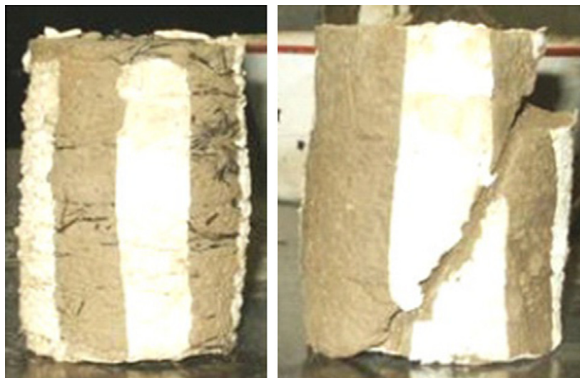
Fig. 2. Specimen deformation pattern for (left) unreinforced clay soil specimens and (right) clay soil reinforced with 0.25% PP of 19 mm: Freilich et al. [99].
